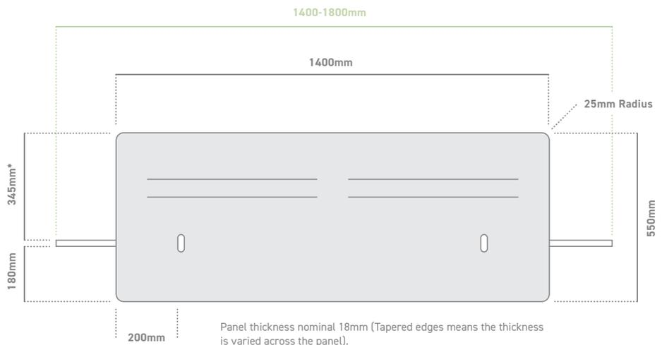
Panel thickness nominal 18mm (Tapered edges means the thickness is varied across the panel).
