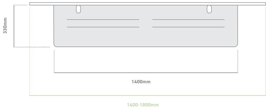
Black mounting brackets screw fix to the underside of the worktop.
